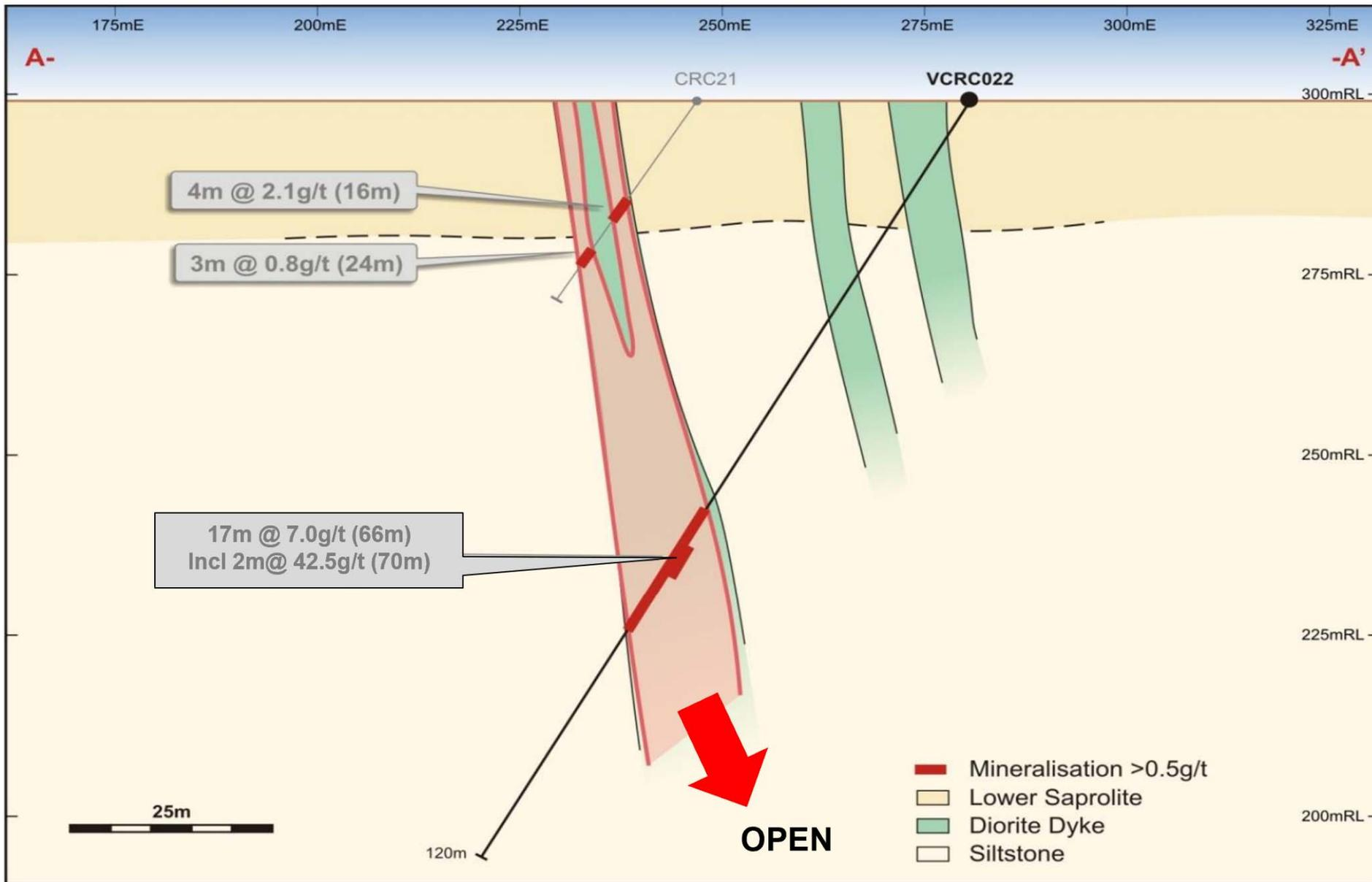
Figure 5: Cross section B-B' (refer to Figure 3) from Clonbinane (modified after Beadall 2008).
