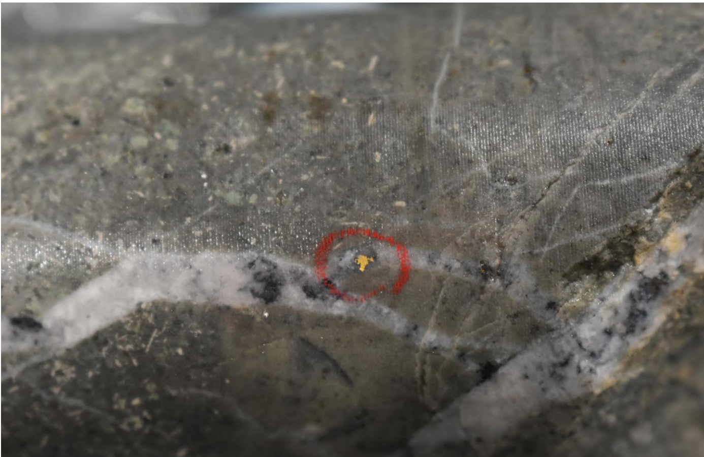
Photo 3: SDDSC064 between 890.2-890.7 m showing visible gold within a quartz carbonate vein stockwork hosted by albitized and sericitized dioritic dyke. Minor fuchsite (lime green) alteration in dyke. Field of view 30mm.
