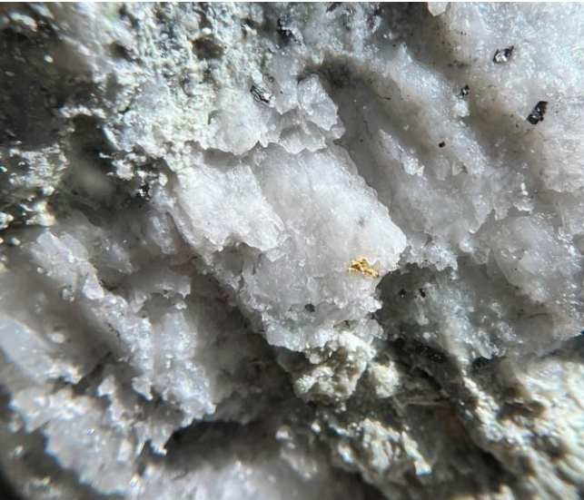
Photo 3: SDDSC049 212.4m, field of view 60mm, showing visible gold in yellow circles within quartz, carbonate and stibnite vein with altered dioritic dyke on margin of vein.
