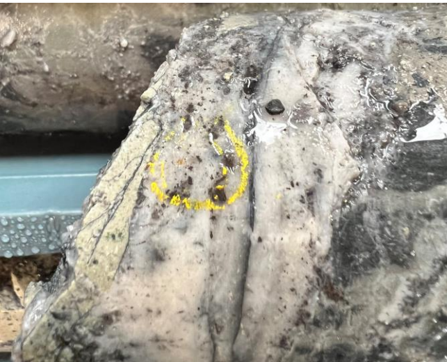
Photo 3: SDDSC049 212.4m, field of view 60mm, showing visible gold in yellow circles within quartz, carbonate and stibnite vein with altered dioritic dyke on margin of vein.
